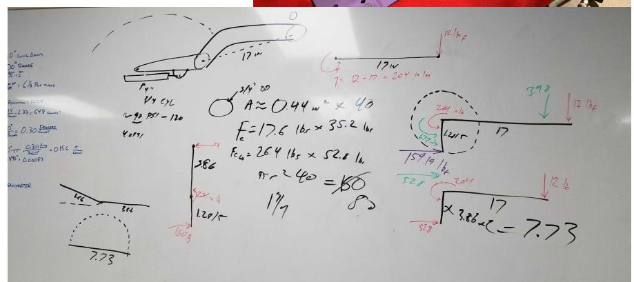
**Motor Pivot Power Solution:** Once we realized that our current solution was way underpowered, and there was no way to step up the bore size of the cylinders in order to gain more force into the system because of packaging constraints, we
