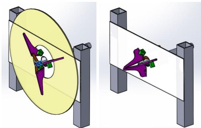
**Scissor Style Grabber**: One of the most promising tests was with a scissor style grabber. This mechanism could grab and release with one actuation. When the hatch panel was held, it was very secure and could not be pulled off. The prototype would need to be more refined in order to fit within the confines of the robot.
