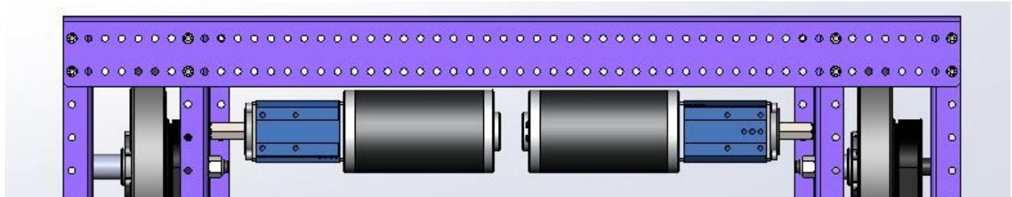
We ultimately decided that this solution would not quite fit our needs. Knowing we wanted to keep the 2x2 box tube towers between the drive rails, and mount the gearboxes between them, servicing these gearboxes was going to be a challenge. We also noted that these gearboxes are rated for 140 ft/lbs, and we would be putting nearly 190ft/lbs through them in a worst case scenario. We investigated a combination of these with an external gear pair, but they too did not fit.
