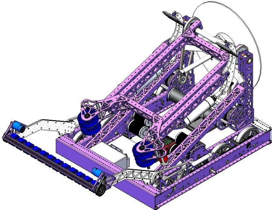
Initial testing of the mechanisms individually was really promising. Each system worked very well independently; the OTB intake could easily acquire balls from the floor and bring them up the bumper without issue, and the rollers on the HAB3 arm could easily acquire and release the Cargo ball. The HAB3 roller set also had plenty of grip on the Cargo ball so that it would not be dropped when traversing the field or moving the arm.
