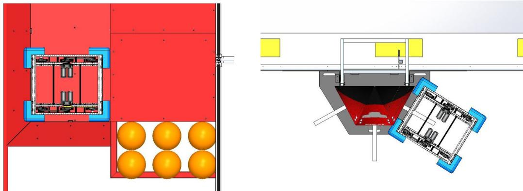
The only concern was alignment with the front face of the cargo ship. With the robot centered on the bay opening, the robot overhangs past the centerline. This would keep two robots from scoring at the same time. This issue was not a big enough deal to change the drive, but just leave as a note to the hatch group for consideration while they completed their designs and strategy.
