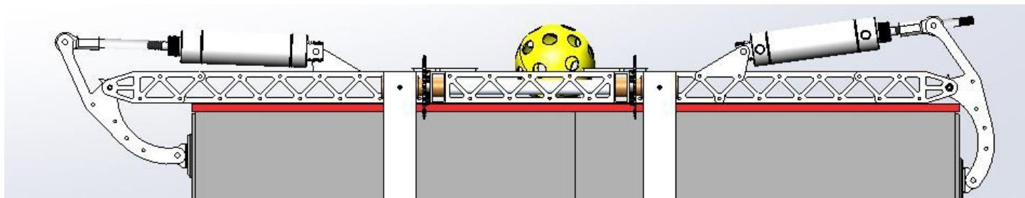
This geometry worked. It allowed for about 3 inches on either side for misalignment room, and still allowed us to grip. Because of the safety factor we built in, we could also ignore some of the weird force vectors that become present when put into a real life scenario with the forces not quite perpendicular to the clamp devices.
