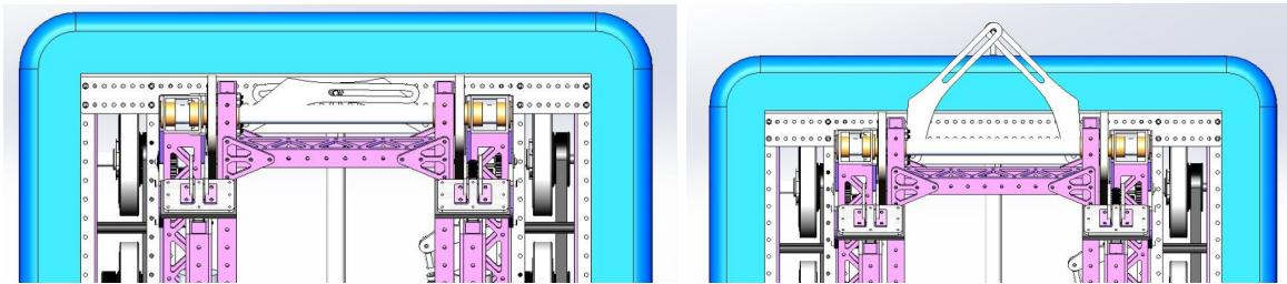
One major issue with this design was that when holding a Hatch Panel, the arms would stick outside of a frame perimeter. By rule, this would keep the team from being able to start a match while holding a panel with this mechanism. To resolve this issue, the team decided on an alternative holder for during the Sandstorm period.
