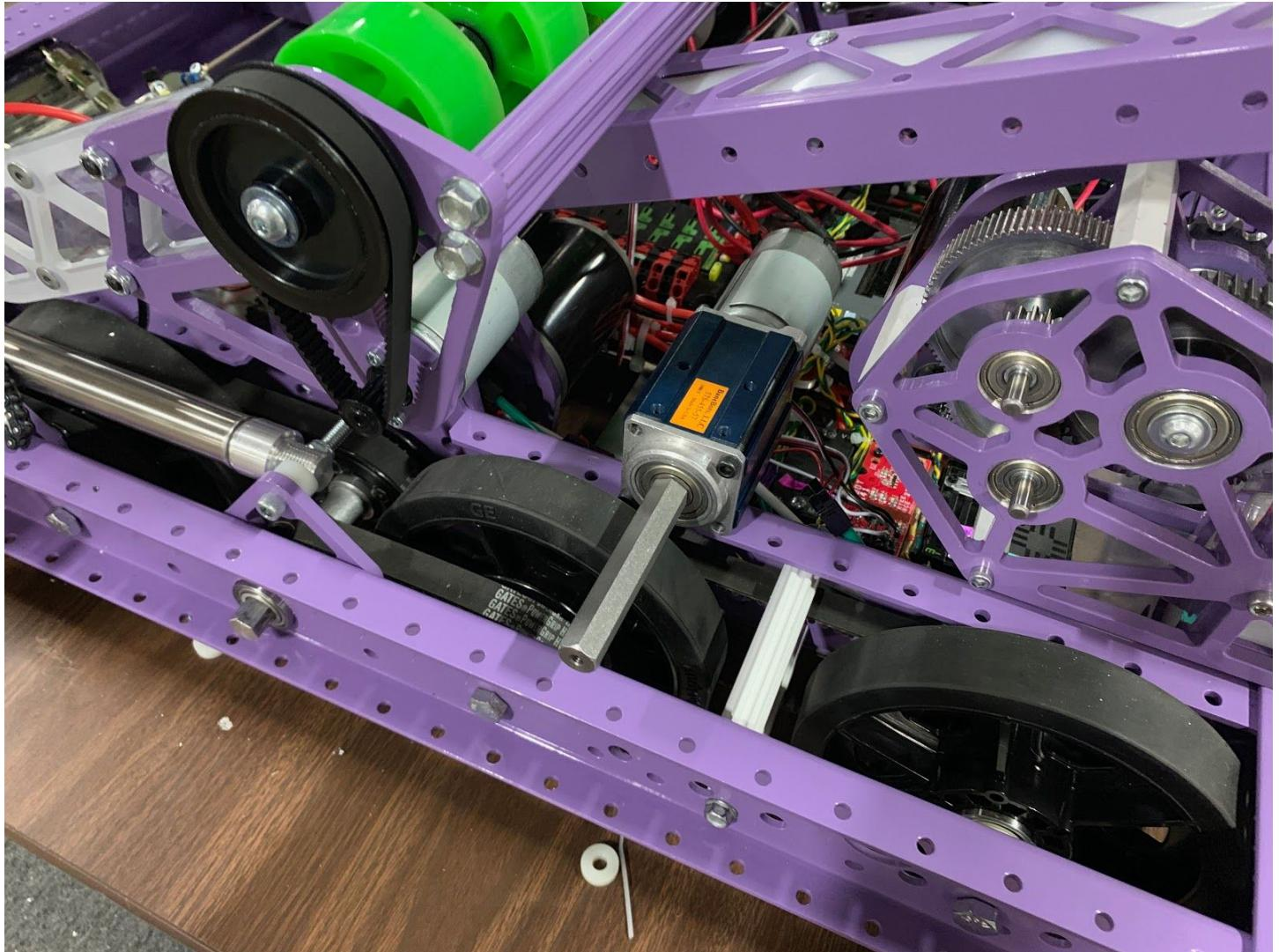
This solution worked out great, and was actually a minimal resource token usage solution too. We also integrated some hall effect sensors at the ends of travel for the mechanism, and essentially treat it like a two position system - it drives each direction until the magnet trips the hall effect sensor, which tells the robot to stop driving the motors.
