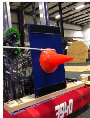
**Edge Grabber** - This group played with different shapes and sizes of parts that can hold onto the hatch panel. One of the largest concerns with this group was ensuring that the hatch panel could be held securely. Early tests with one tab on the inside did not hold as well as multiple contact points. The final iteration of this concept included a concave white spacer securely held the center of the hatch.
