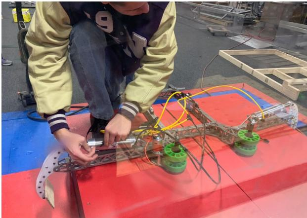
The testing was successful and the grip was enough to support our mentor, Nick standing on the edge of the arm to simulate the weight of the robot cantilevered off the edge of the platform. Although, we understand there would be some variability between this test and final robot operation, the success gave us the confidence to move forward with the design without making major changes.
