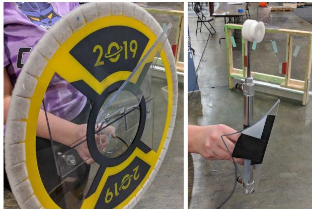
**3 Prong Grabber**: This idea was mocked-up in CAD. It features 3 fingers that reach inside the hatch panel center circle and expand to hold in the center. Being made up of small precision parts this design was hard to make by hand and was created in CAD.
