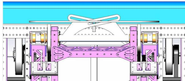
Initially the design called for a 4-arm layout in two layers. This provided a good hold on the hatch panel in prototyping. Unfortunately, this design interfered with the vision system on the robot and required a switch to a 2-arm design.
