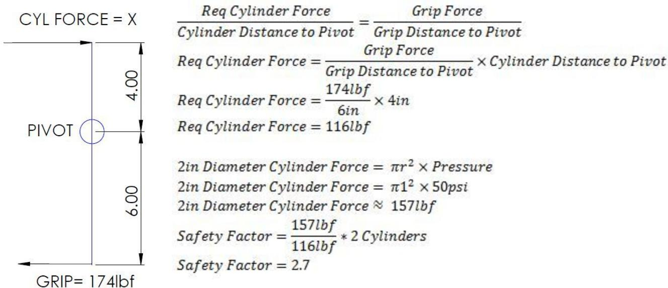
This concluded that we can use 2" bore cylinders and have enough grip strength to curl the robot. We estimate our safety factor is big enough to deal with the shock loads that the grip mechanism may see during climbing sequences. We now need to check if this geometry can allow for enough misalignment (approximately +/- 3" on either side):
