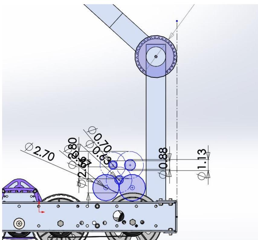
This crayola CAD sketch shows that the gearbox would be compact enough to fit in our desired location of in front of the vertical supports of the arm, as low to the ground as possible to keep the Center of Gravity of the robot low.
